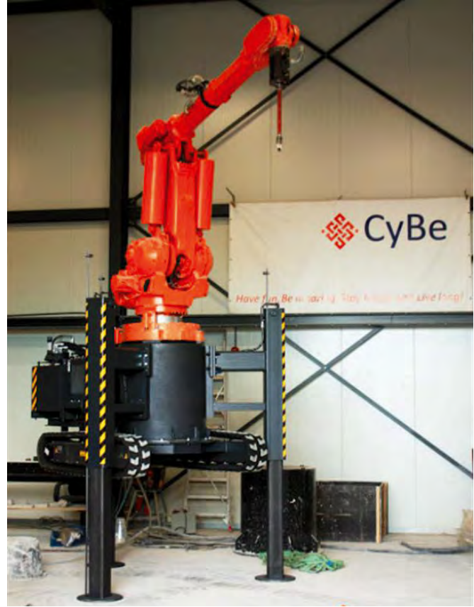
CyBe RC 3Dp mobil beton 3D yazıcı
