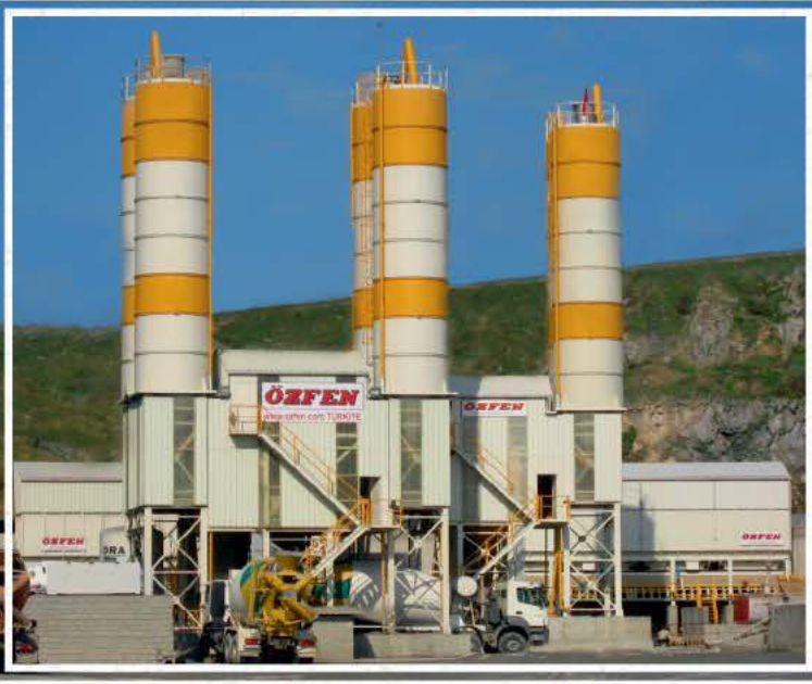
90 m 3 /saat, 120 m 3 /saat BETON SANTRALLERİ MARMARAY / KADIKÖY - KARTAL METRO HATTI
