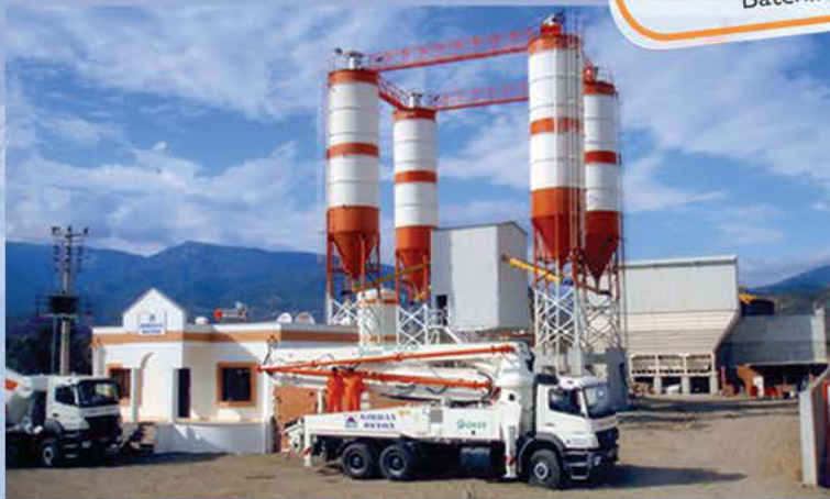
30m³'ten 300m³ kapasiteye kadar sabit beton santralleri Stationary Concrete Mixing Plant capacities of 30 to 300m³/hour
