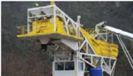
Concrete Batching Plants
