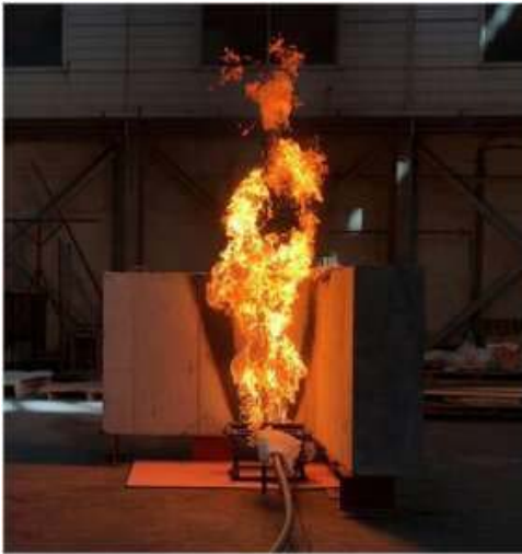
(a) Damaging to concrete by fire
