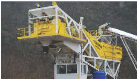
Concrete Batching Plants
